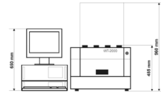
Front view WAF-SCAN System (height 960 mm with front lid open for loading/unloading)
